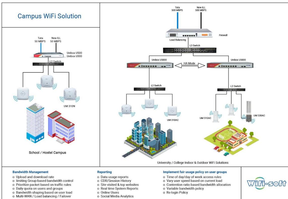
The network deployment will consists of UniBox controller running on a bridge wireless network. The access points can be deployed in various places within the network to provide WiFi coverage to the given geographical area. Each access point will be configured in bridge-mode and will be primarily responsible for relying the traffic back to the controller for authentication and accounting.
