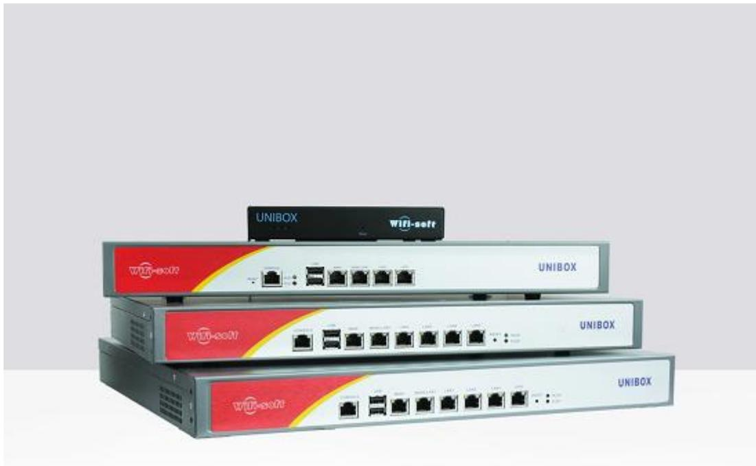
It encompass various functions including hotspot controller/gateway, RADIUS Server, Captive Portal server, URL logger, Web Filtering server, VPN server and Multi-WAN router. All the functions come integrated in a single GUI thus allowing administrator to easily control and manage the wireless network.
