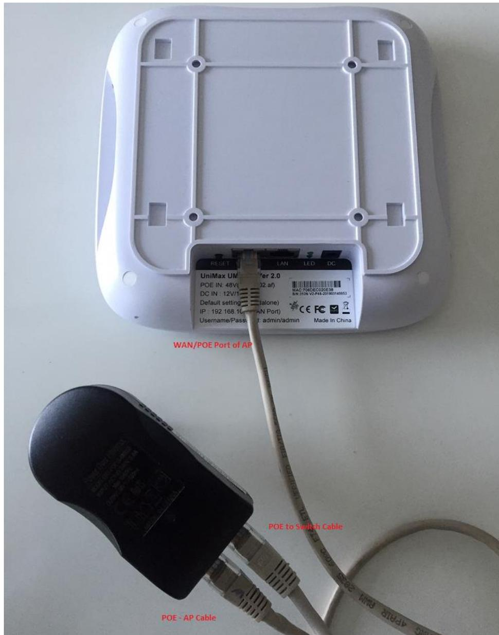
The POE injector has two ports – POE and LAN. The POE port needs to be connected to the WAN port of the access point using a CAT-5 or CAT-6 cable. The LAN port of the POE injector needs to be connected to the switch from where the AP will be get Internet connectivity.
